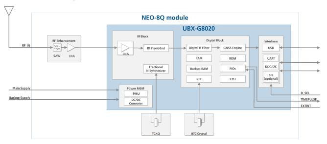
Figure 1: NEO-8Q block diagram
