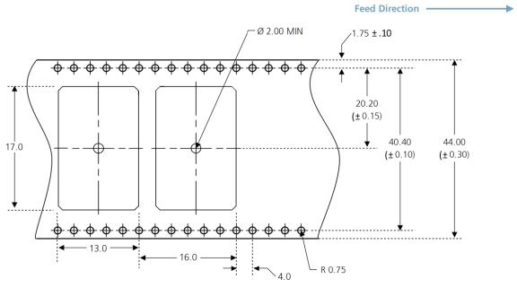
Figure 5: Dimensions and orientation for NEO-8Q modules on tape
