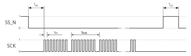
Figure 3: SPI timing diagram
