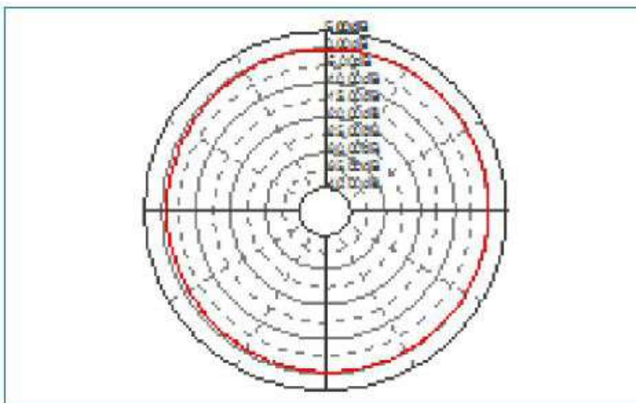
Typical Radiation Patterns for 824-960 MHz frequency band, on Reference Board 50x110mm for yz plane
