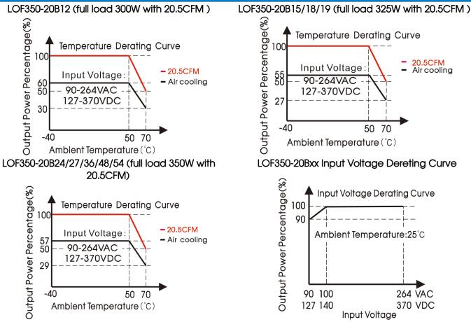
Note: With an AC input voltage between 90 - 100VAC and a DC input between 127 - 140VDC the output power must be derated as per the temperature derating curves.
