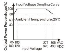
Note: 1. With an AC input between 85-100V/277-305VAC and a DC input between 100-120VDC/390-430VDC, the output power must be derated as per temperature derating curves;
