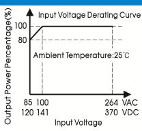
Note: 1. With an AC input voltage between 85-100VAC and a DC input between 120-141VDC the output power must be derated as per the temperature derating curves;
