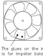
Note: The glues on the impeller is for impeller balance. Please don't remove it.
