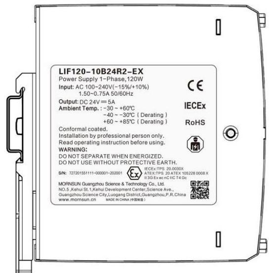
Notice: Keep the following installation clearances: 20mm on top, 20mm on the bottom, 5mm on the left and right sides are recommended when the device is loaded permanently with more than 50% of the rated power. Increase this clearance to 15mm in case the adjacent device is a heat source (e.g. another power supply).
