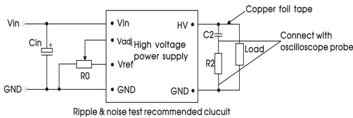
Ripple & noise test recommended circuit
