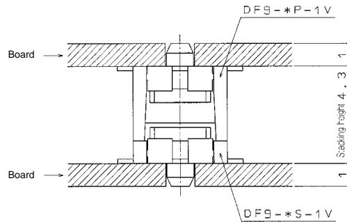
Note 1 : The board to board size 4.3mm in the pattern does not include the soldering paste thickness.
