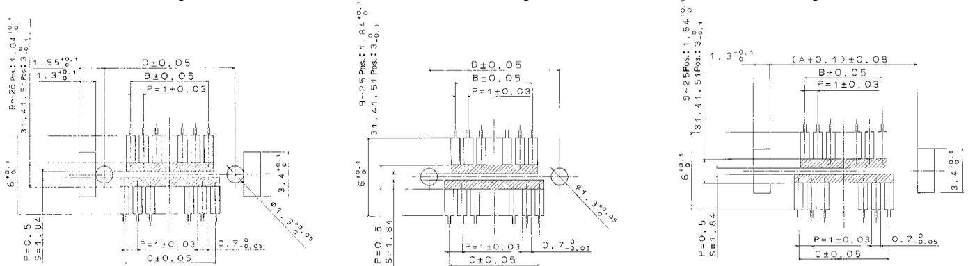
Note 1 : If the pattern is included in the shaded area and not treated with resist, it could touch the connector contact .
