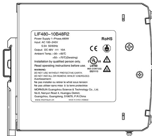
Note: Keep the following installation clearances: 20mm on top, 20mm on the bottom, 5mm on the left and right sides are recommended when the device is loaded permanently with more than 50% of the rated power. Increase this clearance to 15mm in case the adjacent device is a heat source (e.g. another power supply).
