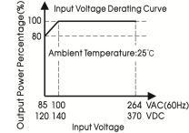
Note: 1. With an AC input voltage between 85-100VAC and a DC input between 120-140VDC the output power must be derated as per the temperature derating curves;
