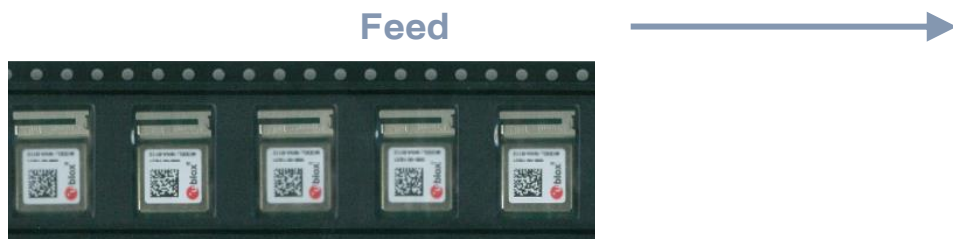
Figure 10: Orientation of NINA-B222 module on tape
