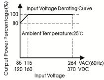
Note: 1. With an AC input voltage between 85-115VAC and a DC input between 120-160VDC the output power must be derated as per the temperature derating curves;
