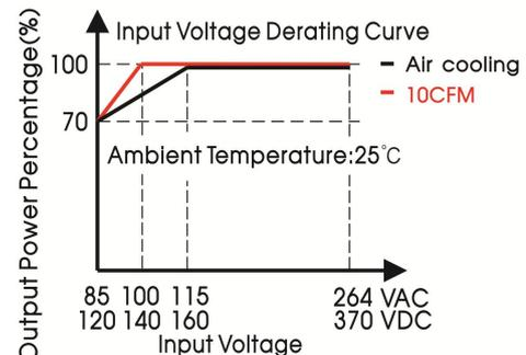
Note: With an AC input voltage between 85 - 115VAC and a DC input between 120 - 160VDC the output power must be derated as per the temperature derating curves.
