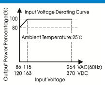
Note: 1. With an AC input voltage between 85-115VAC and a DC input between 120-163VDC the output power must be derated as per the temperature derating curves;
