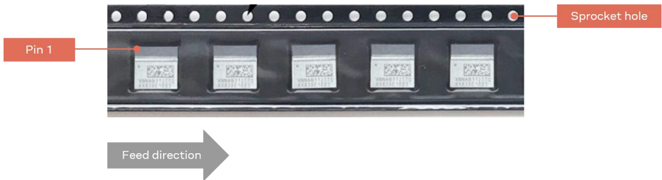
Figure 8: Orientation of ANNA-B4 modules on tape
