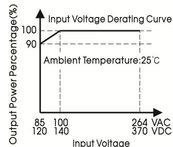
Note: 1. With an AC input voltage between 85 -100VAC and a DC input between 120-140VDC the output power must be derated as per the temperature derating curves;
