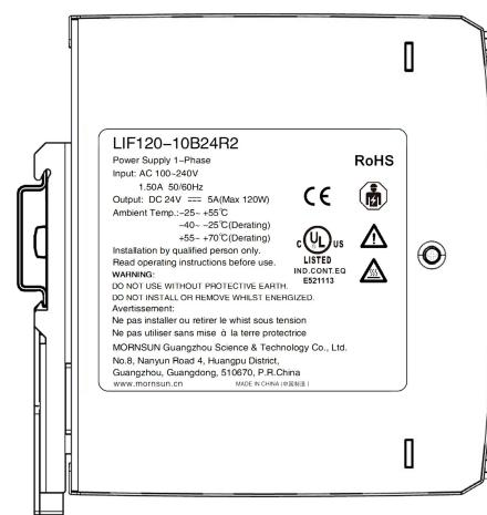
Note: Keep the following installation clearances: 20mm on top, 20mm on the bottom, 5mm on the left and right sides are recommended when the device is loaded permanently with more than 50% of the rated power. Increase this clearance to 15mm in case the adjacent device is a heat source (e.g. another power supply).
