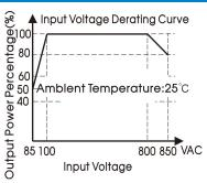
Note: ① With an input between 85 - 100VAC/800 -850VAC, the output power must be derated as per temperature derating curves;
