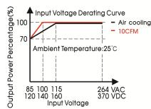
Note: With an AC input voltage between 85 - 115VAC and a DC input between 120 - 160VDC the output power must be derated as per the temperature derating curves.
