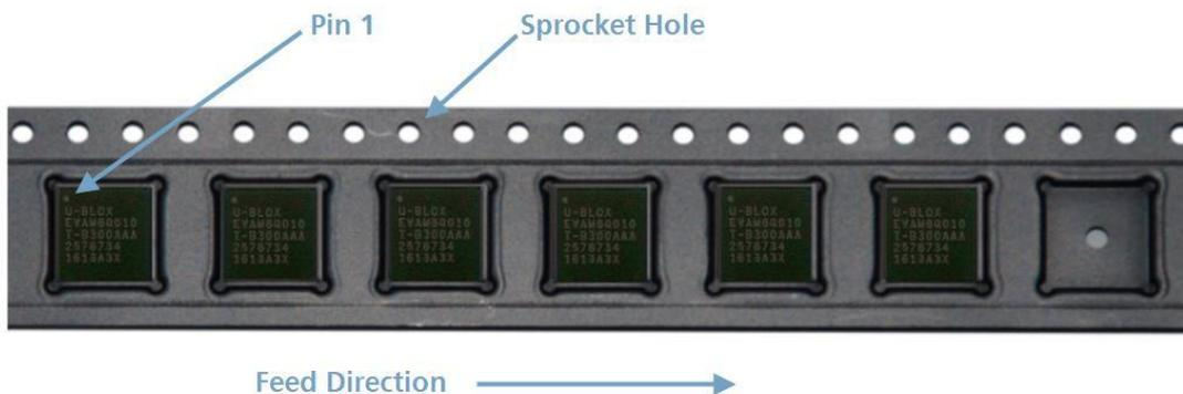
Figure 6: Orientation of EVA-M8M/Q modules on the tape
